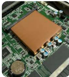
Copper heat sink cooling system
